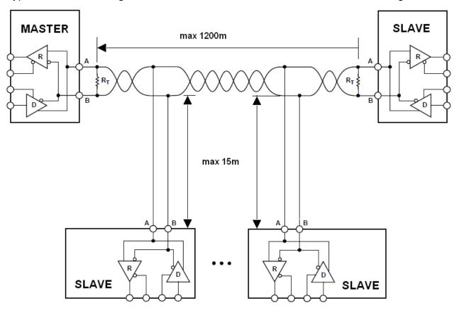
Figure 2. Connection diagram of two-wire RS485 bus
