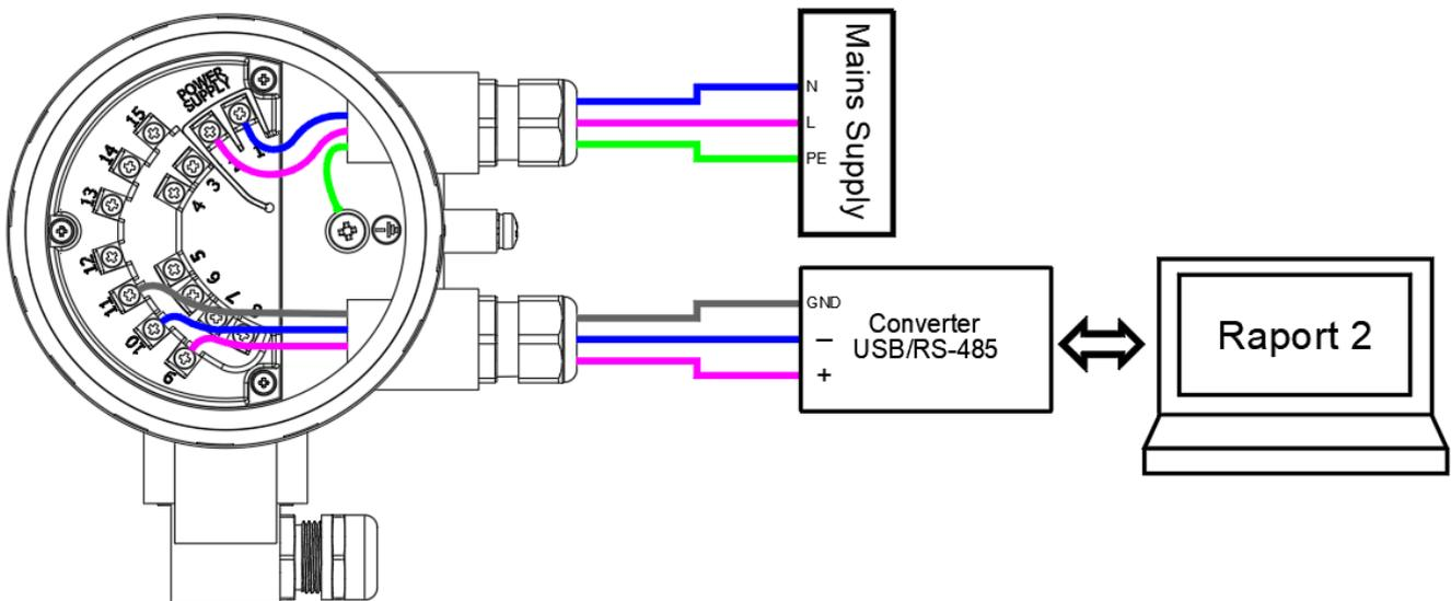
**Figure 23.** Connection using communication and mains supply
