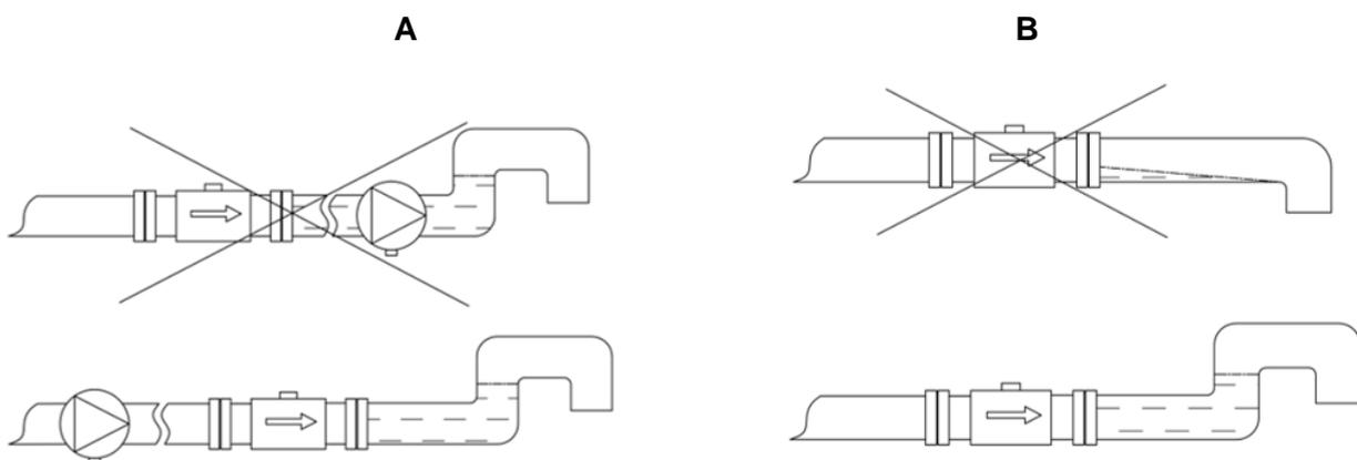
**Figure 5.** Examples of incorrect sensor installation on the site and suggested solutions
