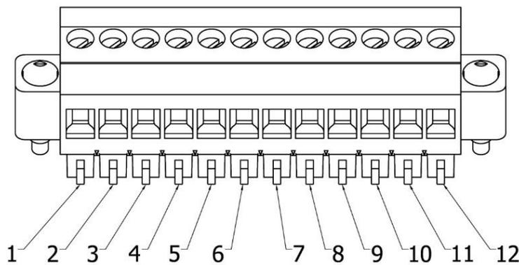
**Figure 11.** Connection pins of the sensor cable plug
