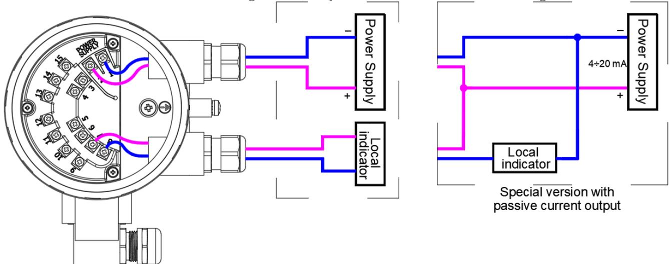
**Figure 20.** Connection using an analog current output of 4...20 mA and low-voltage power supply
