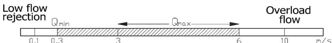
**Figure 24.** Recommended flow values of the PEM-1000 flowmeter
