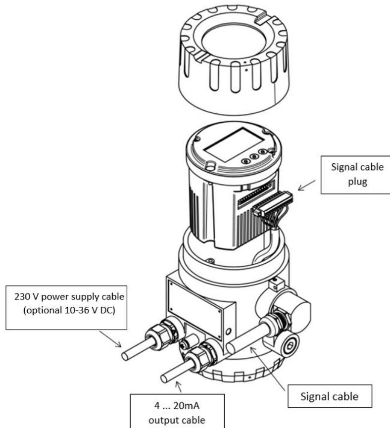
**Figure 8.** Electrical wiring from the PEM-1000 transmitter
