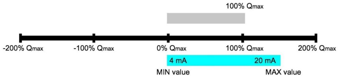
**Figure 25.** The measuring range of the flowmeter is determined by the Qmax parameter
