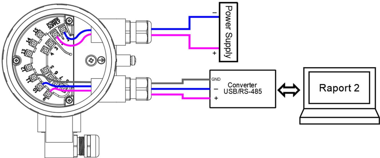
**Figure 22.** Connection using communication and low-voltage power supply
