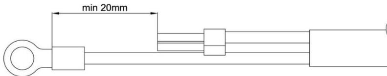
**Figure 15.** Proper preparation of the power cable
