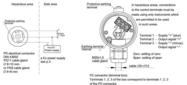
Figure 3. Connection of the transmitter with PZ electrical connectors.
