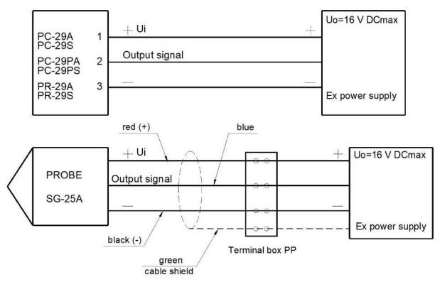
Figure 1. Power supply PC-29A, PC-29S, PC-29PA, PC-29PS, PR-29A, PR-29S, SG-25A with a "linear" characteristic - example.
