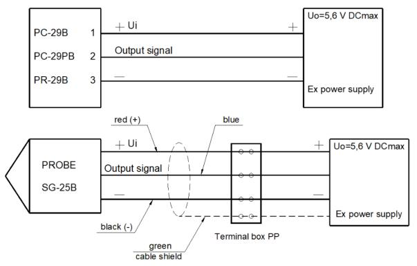
Figure 2. Power supply PC-29B, PC-29PB, PR-29B, SG-25B with a "linear" characteristic - example.
