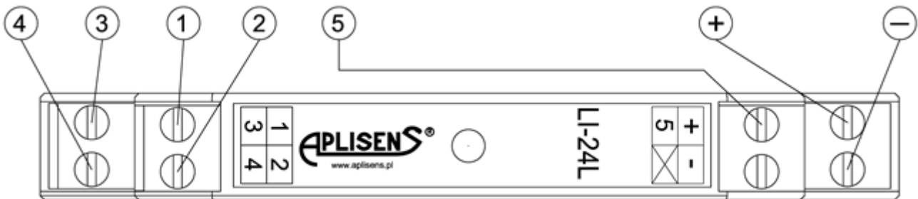
Figure 8. Markings of LI-24L transmitter terminals.
