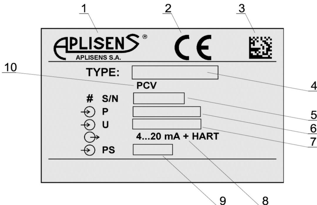
**Figure 2.** APRE-2000GN transmitter nameplate.
