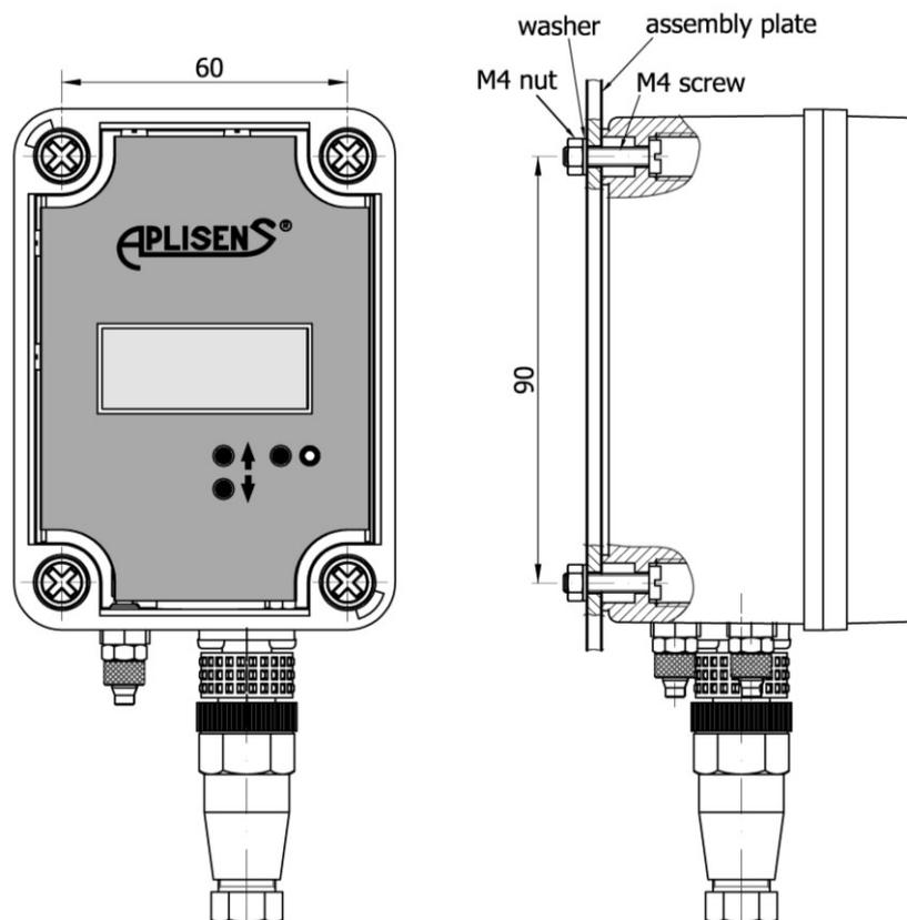
Figure 4. **APRE-2000GN** differential pressure transmitter – mounting method.
