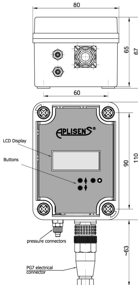
**Figure 3.** APRE-2000GN differential pressure transmitter – dimensions.
