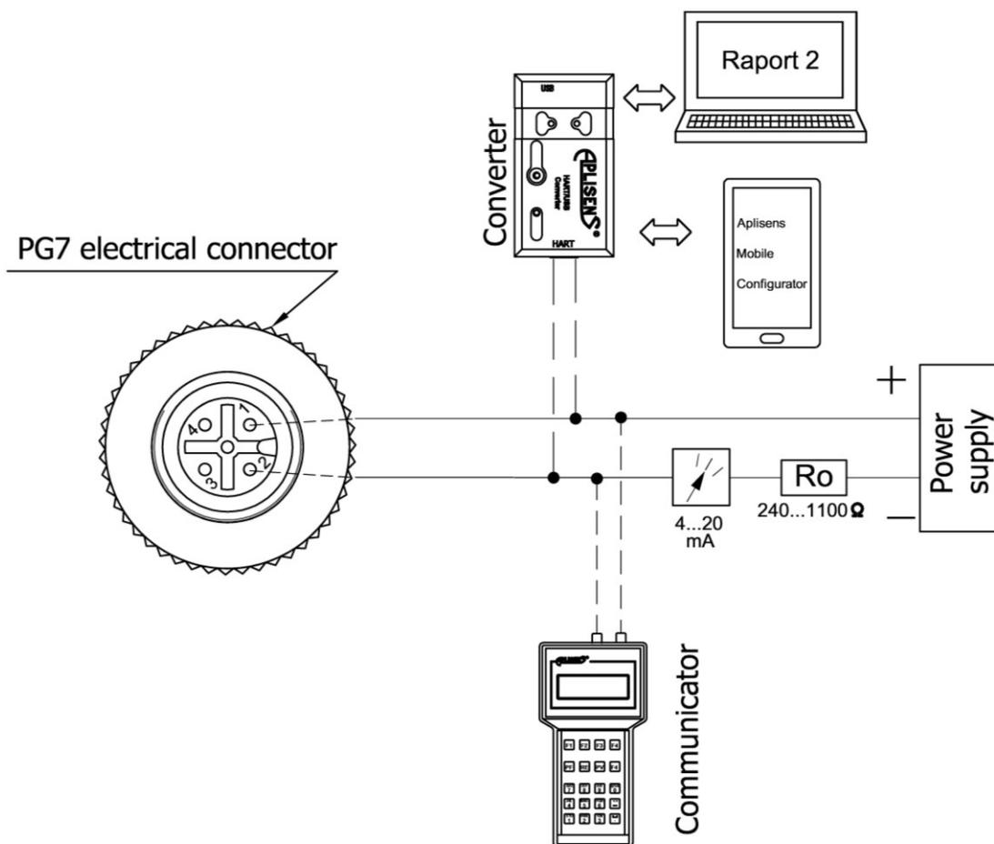
**Figure 5.** Connection of the **APRE-2000GN** transmitter and communicator or modem.
