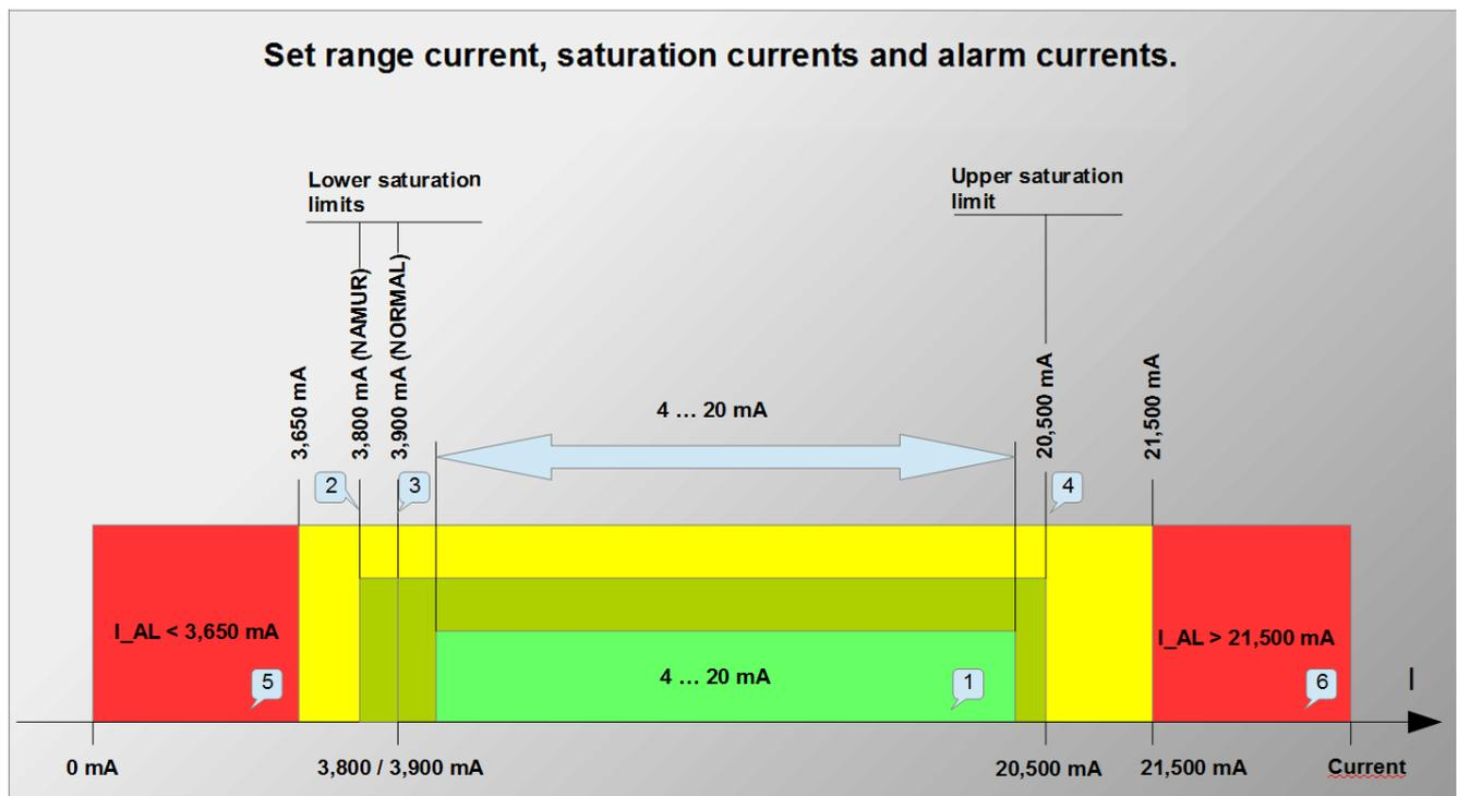
**Figure 7.** Set range current, saturation currents, alarm currents.
